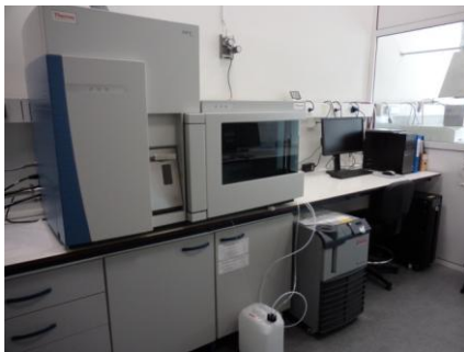
Inductively Coupled Plasma Mass Spectrometry (ICP-MS, Thermo ICAP-Qc)
