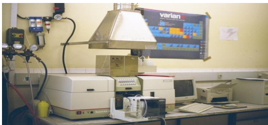
Flame Atomic Absorption Spectrometry (Varian SpectrAA 200)
