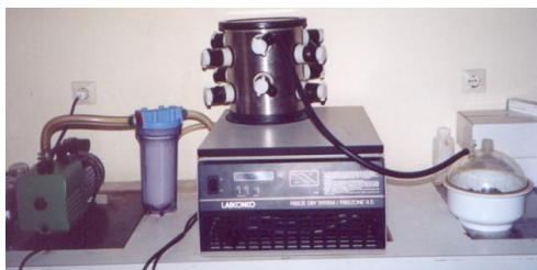
Freeze dryer (Freezone / LABCONCO)
