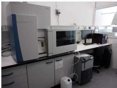
(Inductively Coupled Plasma - Mass Spectrometer, Thermo ICAP-Qc)
