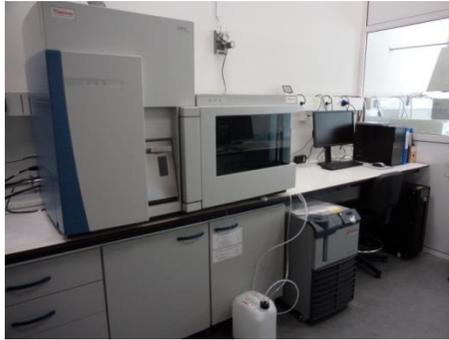
(Inductively Coupled Plasma - Mass Spectrometer, Thermo ICAP-Qc)
